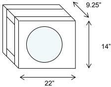
Two Woofers, Sealed Box. Net Internal Volume per side: 1 ft<sup>3</sup>
