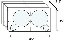
4th Order Band-Pass. Sealed Net Volume: 0.55 ft3, Ported Net Volume: 1 ft3, Fb: 66 Hz
